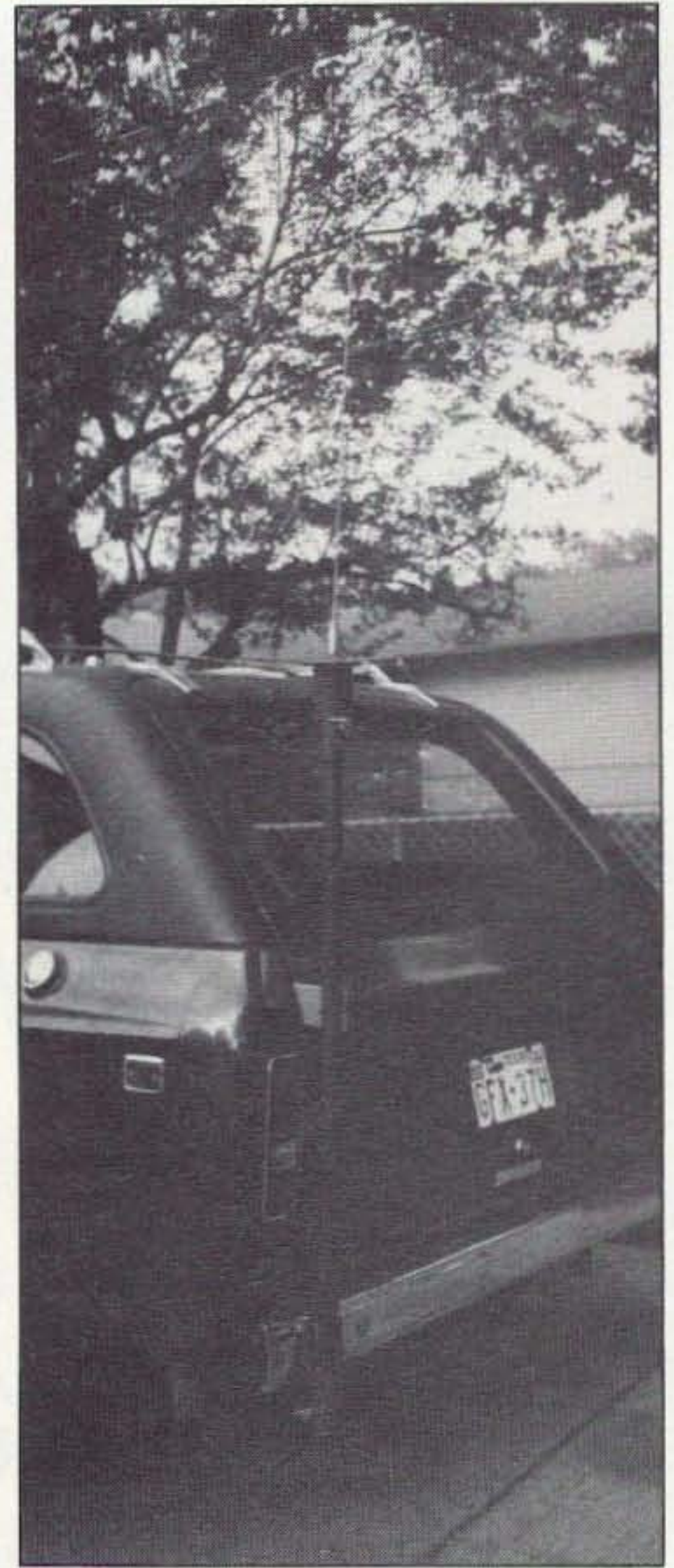
Photo C. 20 meter resonator mounted on the mobile mast.
